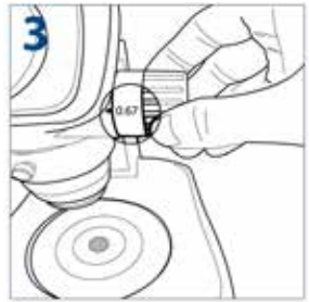
Turn the zoom adjustment knob to the lowest magnification
