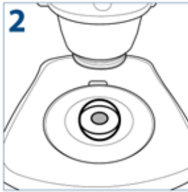
Put a specimen on the stage plate
