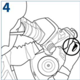
Rotate the focusing knob to bring the specimen into focus
