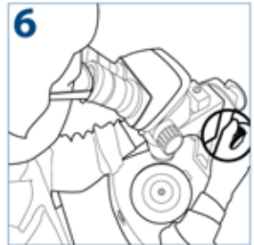
Rotate the focusing knob to bring the specimen into focus
