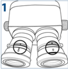
Turn the diopter adjustment rings of both eyepieces to position "0"
